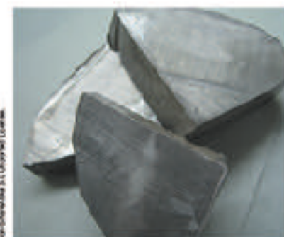
In its pure form, the element sodium is a silvery metal. Its atoms share their mobile electrons and are held together by metallic bonds. It is a very reactive metal.
