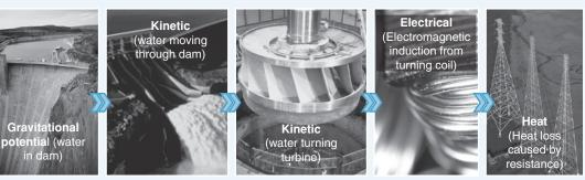
An energy chain can be used to describe where the energy used to generate electricity comes from (and goes to). The number of steps in the chain depends on the form of energy being used and the type of energy generation.
