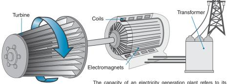
The capacity of an electricity generation plant refers to its instantaneous power output. For example, a plant rated at 1000 MW has the ability to produce 1000 megawatts (1000 megajoules per second) of electricity at any one point in time.
